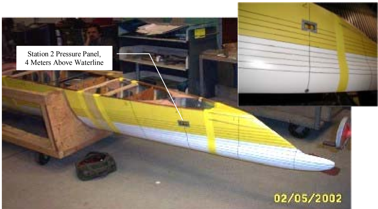
Figure 5. Starboard Bow View of Station 2 Pressure Panel and Keel Pressure Transducer
