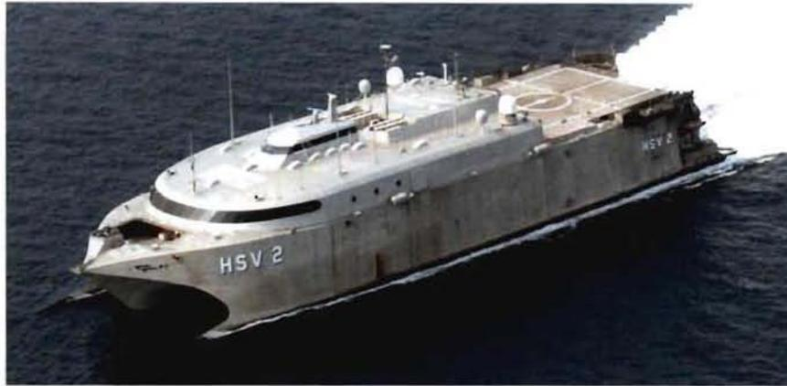
**Fig. 1:** All aluminum high-speed vessel *HSV-2 Swift*
