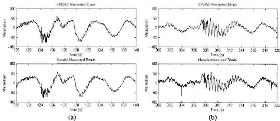
**Fig. 10:** Strain response on SeaFighter Frame 20:
