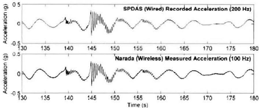
Fig. 11: Acceleration response of the *SeaFighter* measured at the center of gravity.
