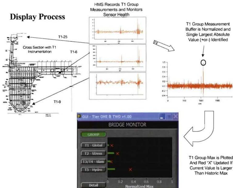
Fig. 6: Example of measurement and information display
