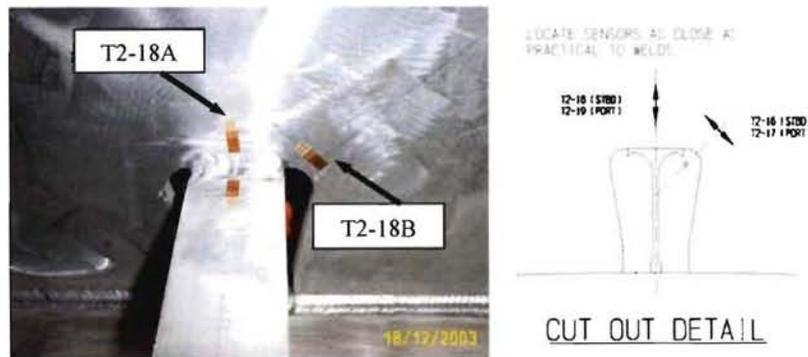
**Fig. 2:** Examples of local high stress T2 A-B pair strain gages
